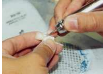
The bulk of the refractory is removed using a diamond.
