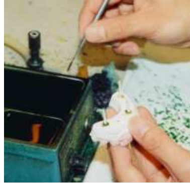
After the pins are glued with the Z-20 Spacer, a small amount of wax is added to prevent sticking to the base.
