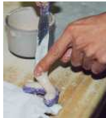
Before the initial set the refractory will thicken allowing it to be stacked.
